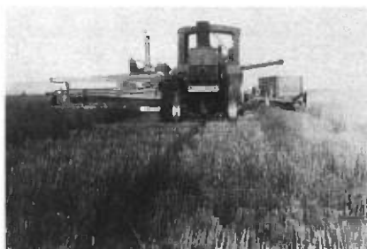
First mechanical combine in Ford County. It harvested the grain standing and put it in the wagon behind.
