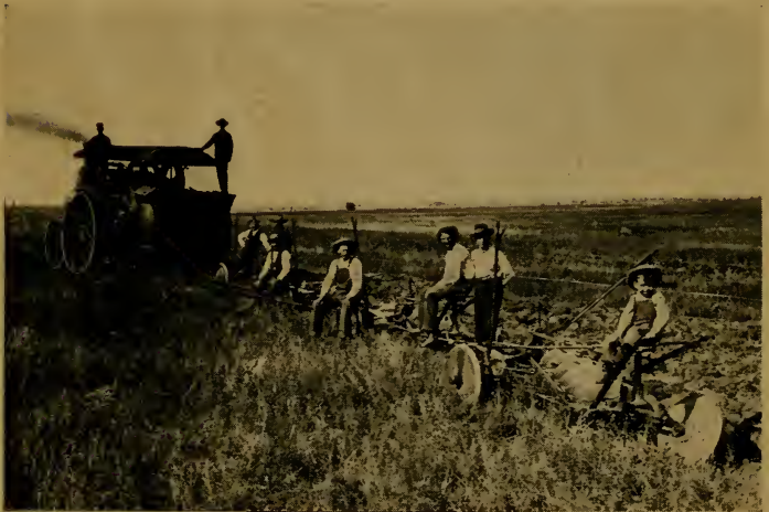
Twenty-four disc, steam plow, owned by Wm. Morris, Graham county. (4 rigs in county.) Cuts 4-inch sod, 16 feet to swath, turns 40 acres per day, and consumes 1\frac{1}{2} tons of coal.
